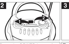
Press the POWER button **1** to the in position and slide the Function switch **2** to select CD; the POWER indicator will light.
